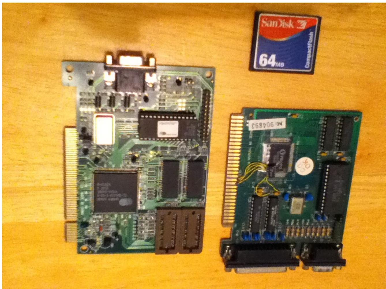
Notes: Peripheral cards provide a way of adding capabilities to the system; There is a variety of busses for peripheral cards, the image shows – ISA, PCI and Compact Flash cards
